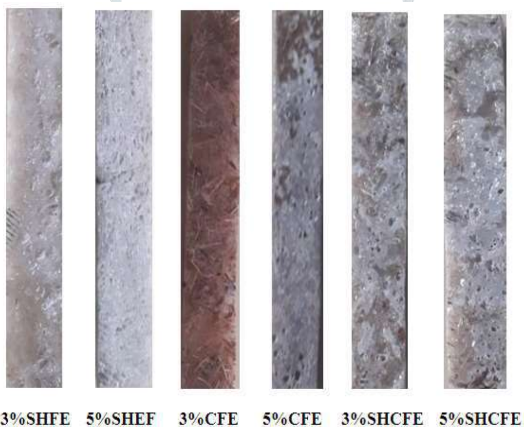
Fig. 5 Specimen prepared with different combination of reinforcement and matrix material
