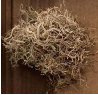
Fig.2 Munja fibre of 15 mm length.
