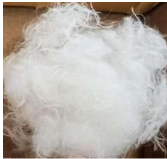
Fig 3. Polypropylene fiber of 15 mm length.
