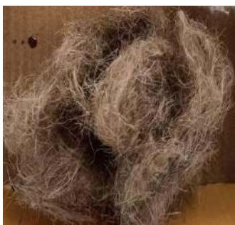
Fig.1 Jute fibers of 15 mm length.
